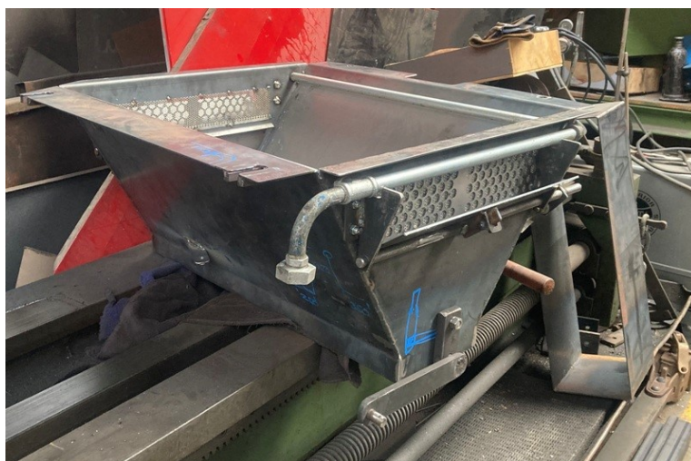
Photo showing the ashpan all complete ready to be fitted up.
