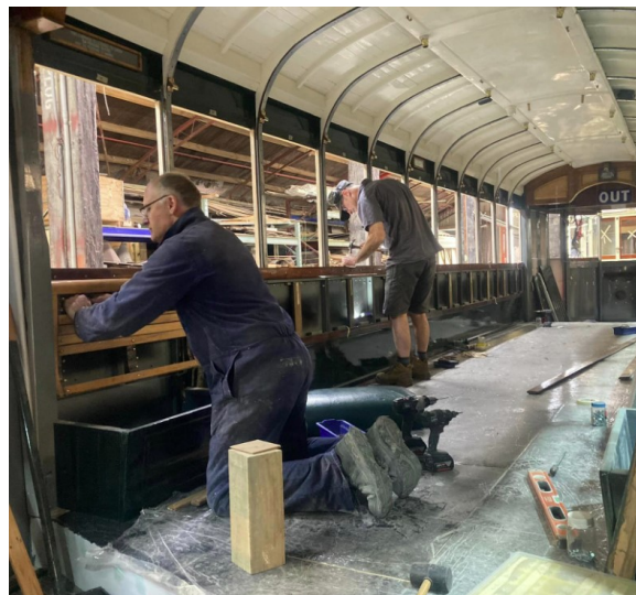
Graeme and Leighton fitting up seats and interior walls.
