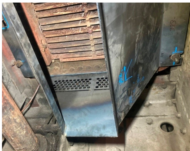
Photo Showing the ashpan in place for a trial fit.
