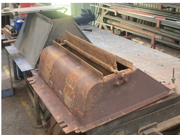
Photo above - showing the old and the new ashpans during the construction of the new one.
