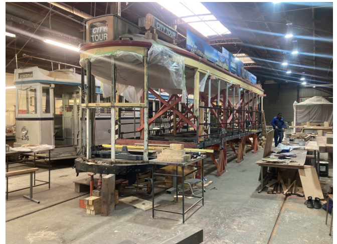
178 at present, by the next issue of tracts it should have sides fitted on.
