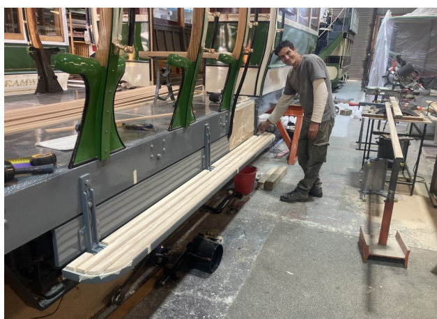
Shay fitting the step slats, these are a real work of art.
