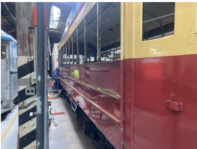
The offside nearly completely stripped and revealing many points of rot and corrosion.
